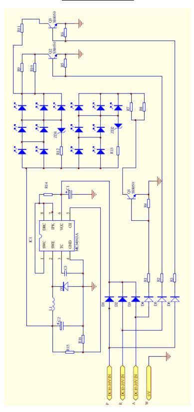
Non-replaceable light source (Input range: 10V - 30V) Stop and rear position lamp: 7LEDs, 12V 1.4W/0.4W Rear direction indicator: 7LEDs, 12V 1.3W
